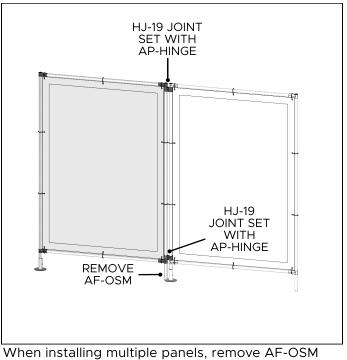
When installing multiple panels, remove AF-OSM from one of the panels to join together. Clip AP-HINGE on top / bottom, assemble HJ-19 joint sets.
