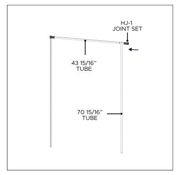
Assemble HJ-1 joint set, 70 15/16" tube and 43 15/16" tube at opposite end.
