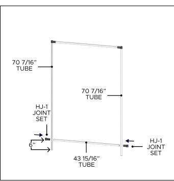
Measure 6" inches from the bottom of 70 15/16" tube, assemble HJ-1 joint set with 43 15/16" tube. Repeat at opposite end with HJ-1 joint set. STEP 2
