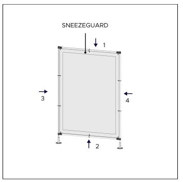
Install Sneezeguard with tie-wraps. start on top, then bottom and finish with sides. Cut excess and turn inward.
