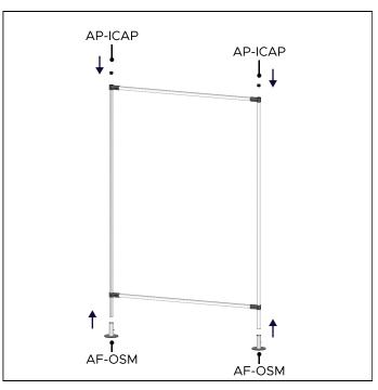
Press-fit AP-ICAP into 70 15/16" tubes. Slide AF-OSM into 70 15/16" tube and secure with F-A85/8 self-tap screw.
