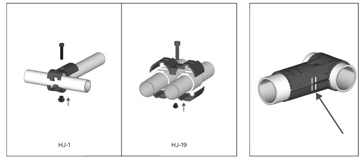
Group connectors around tube and loosely tighten nut and bolt. Insert corresponding tubes and fully tighten with 5mm allen key. Insert smaller diameter of nut into the connector. Feel for thread of bolt throught nut.
