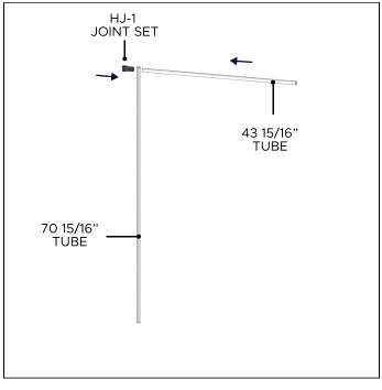
Assemble HJ-1 joint set, 70 15/16" tube and 43 15/16" tube.
